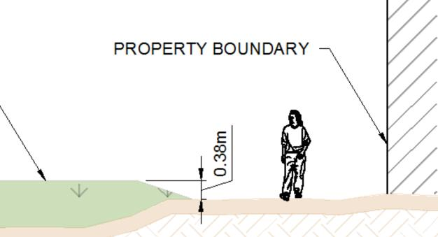
Section B-B: "Gauld's Gas" embankment cross section (sizing for 200 year plus climate change)
