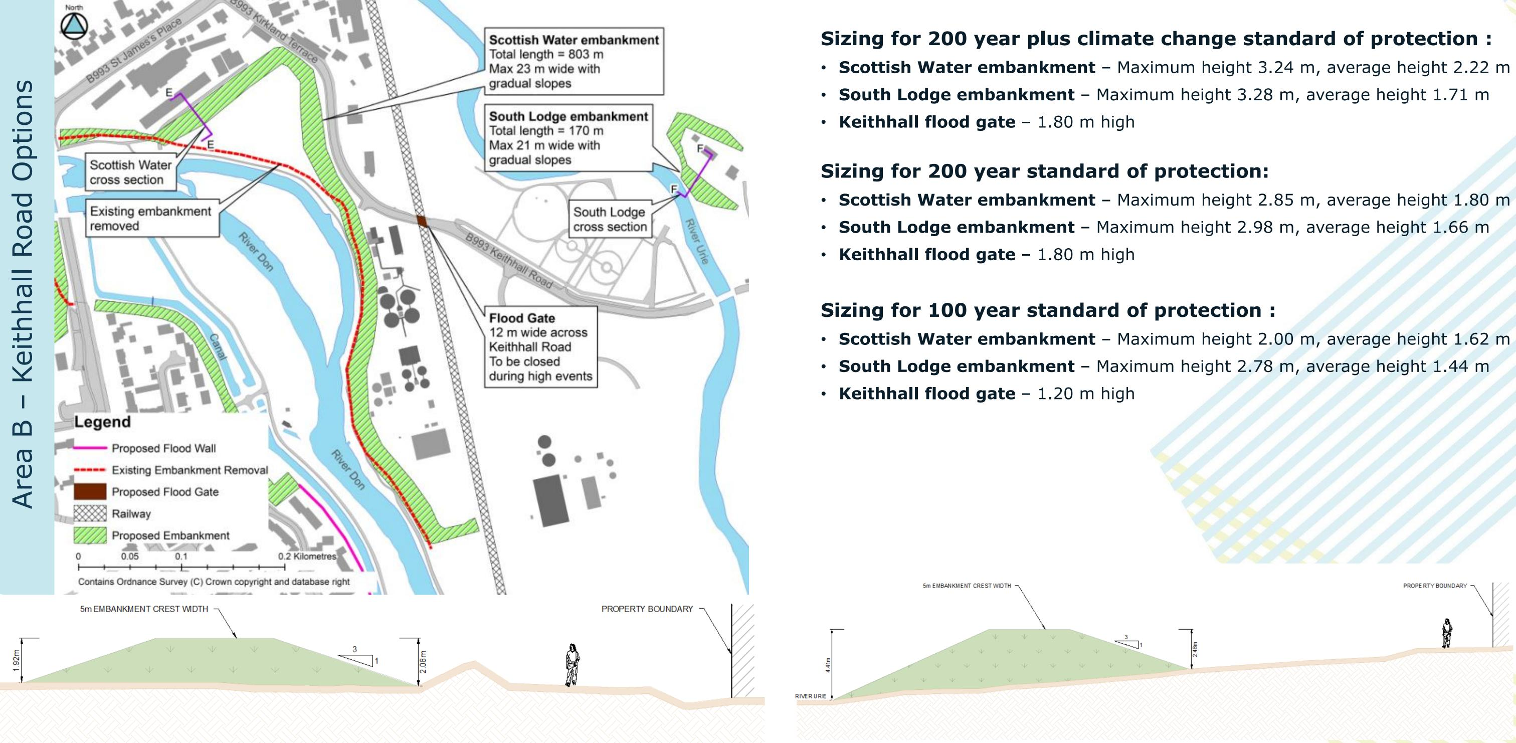
Section E-E: Scottish Water embankment cross section (sizing for 200 year plus climate change)
