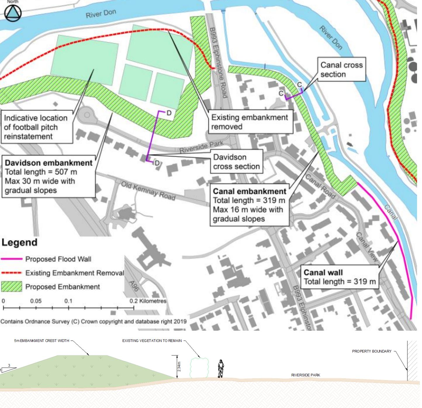
Section D-D: Davidson Field embankment cross section (sizing for 200 year plus climate change)
