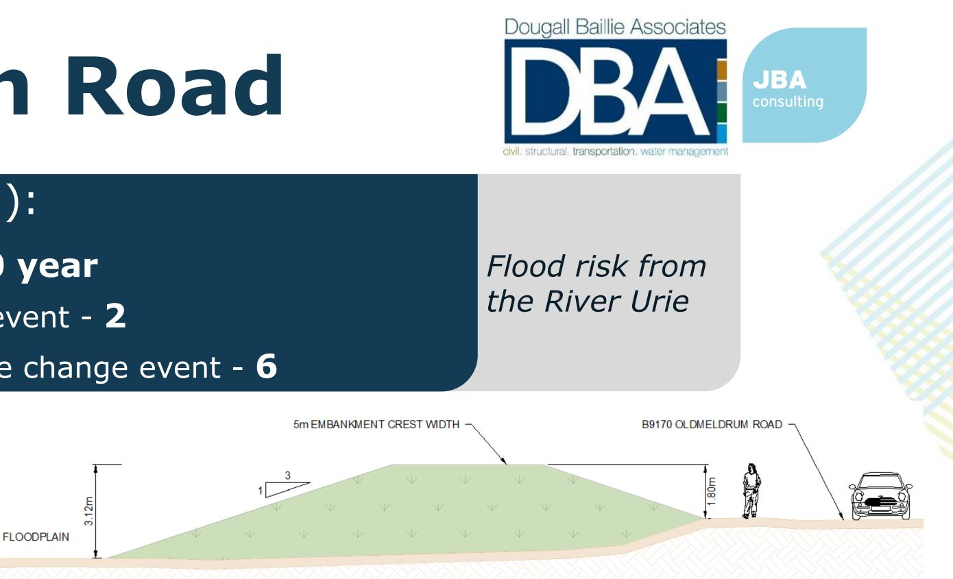
Section A-A: Oldmeldrum Road embankment cross section (sizing for 200 year plus climate change)
